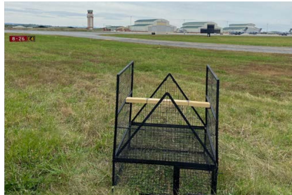
A bird trap made by Airmen in the 167th Maintenance Group's Fabrication Flight sits on the airfield near the 167th Airlift Wing, Shepherd Field, Martinsburg, West Virginia, Sept. 30, 2022. The traps were made to help reduce potential damage and safety concerns posed by the increased number of raptors at the airfield. (photo courtesy of Travis Flanagan, USDA)
