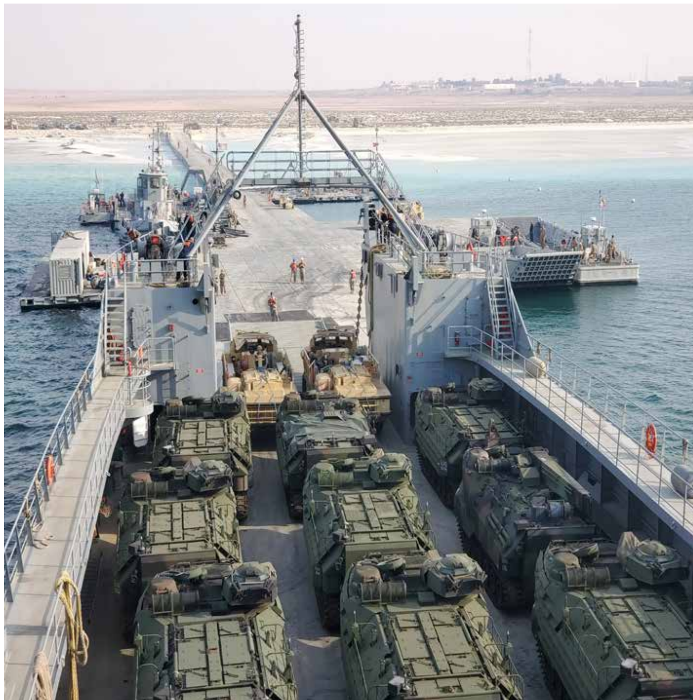
During Joint Logistics Over the Shore Native Fury 21, Soldiers from the 368th Seaport Operations Company alongside the U.S. Navy and Marines download Naval equipment for a training opportunity. The floating platform, or Trident pier, is used for linking deeper drafting vessels to the shore. (Photo by Capt. Jordan Jendersee)
