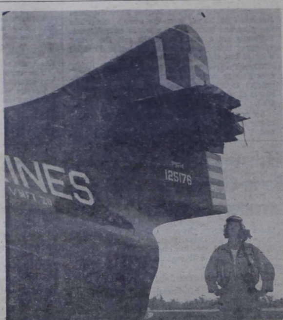
SHAVED TAIL —Second Lt. Kenneth S. Carlson, Marine pilot, takes a look at what is left of the tail assembly of his F9F-4 Panther jet after a mid-air collision with another jet on a routine training mission at Cherry Point last week. After a suspenseful 30 minutes in the air Lt. Carlson managed to land the plane with only slight damage and a saving of $450,000 to taxpayers (Official USMC Photo).
