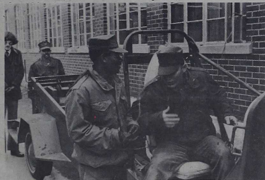
"I'M A BELIEVER!" — Sitting in the "Convincer", a device that simulates the effectiveness of seat belts in a 7 mph collision, LCpl. Mitchell O. Clement comments on his quick stop to Cpl. Ronald Roberts. Both Marines are members of 1st Bn., 10th Marines.
