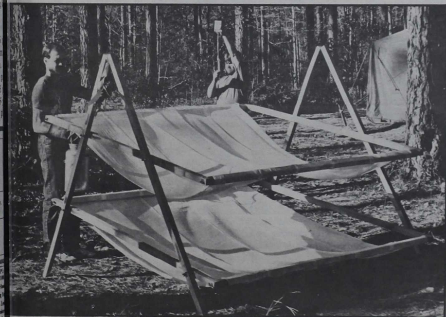
James Jones, engineer technician and Donald Soule engineer mechanic of the U.S. Army Chemical Research and Engineering Center, Aberdeen, Md., spray a chemical net with methyl salicylate, a chemical with the same absorption and diffusion properties as a blister agent but without being harmful. Spraying is part of the operational testing being conducted on the Portable Collective Protective System.
