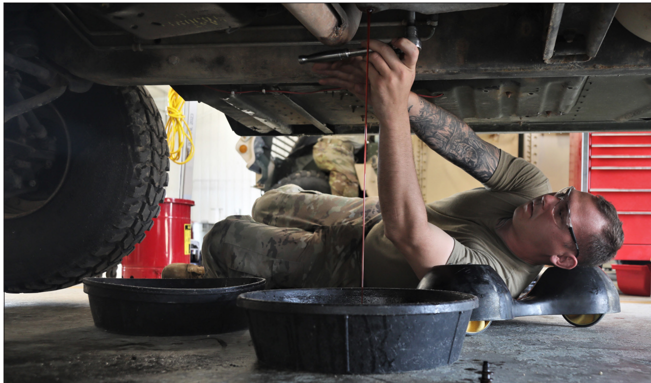
Sgt. Adam Bergelin with the 102nd Military Police Company, Sheboygan, Wis., drains transmission fluid June 15 from a Humvee in order to change the internal transmission filter during Operation Platinum Wrench at the 88th Readiness Division Draw Yard at Fort McCoy.
