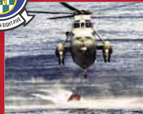
Loading a 324-gallon Bambi Bucket at Lake Miramar, Calif., weighing 3,000 lbs.
