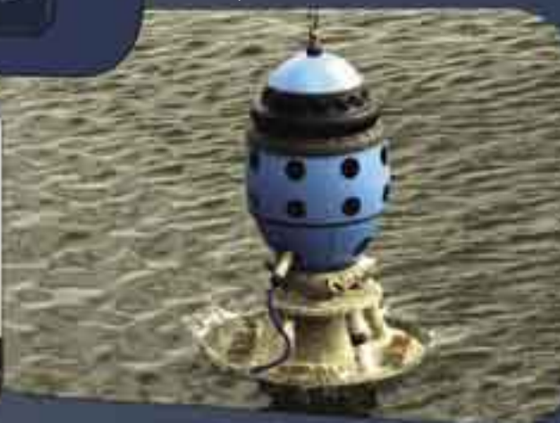
GERBERUS, the acoustic swimmer detection device.
