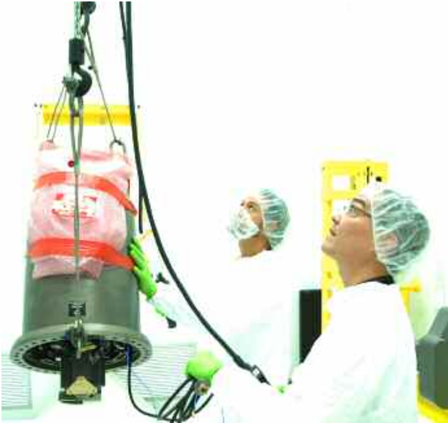
(Left to right): Peter Reimers, code 950 optical instrument repairer, and Jeffrey Uehara, code 950 work leader, prepare a Virginia-class submarine photonics mast’s outer head to remove the optical bench during a phase II photonics validation.
