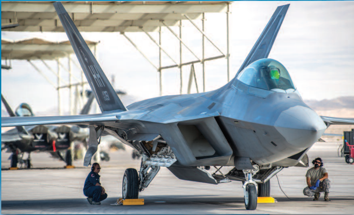
(Left, below) Maintainers deployed from the 15th Wing and 154th Wing, Air National Guard, crew conduct pre-flight checks prior to launching an F-22 Raptor in support of Red Flag 13-2 from Jan. 21 through Feb 1.
