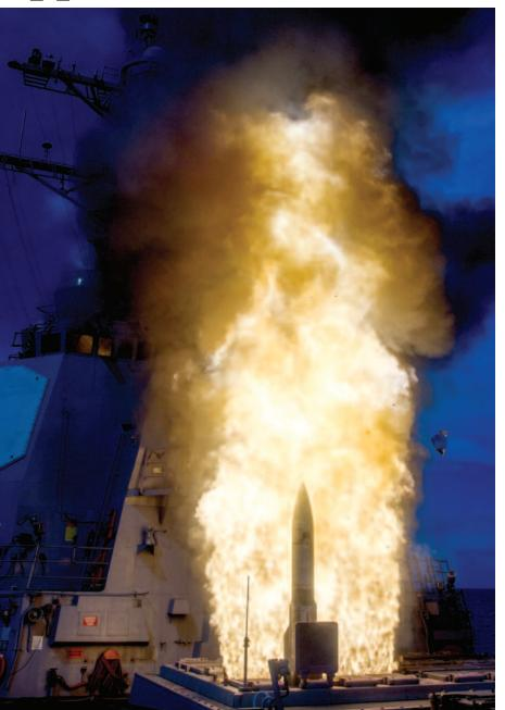
A Standard Missile-2 (SM-2) Block IIIA guided missile is launched from the USS John Paul Jones (DDG-53) during a Missile Defense Agency and U.S. Navy test over the Pacific Ocean by the Aegis baseline (BL) 9.C1 (BMD 5.0 capability upgrade) weapon system configured ship.
