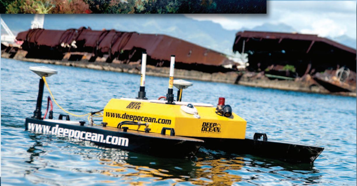
(Right) An unmanned surface vessel from Deep Ocean Engineering conducts multi-beam sonar surveying Oct. 23 at the USS Utah Memorial. U.S. Navy photo by MC3 Johans Chavarro (Below) Technicians analyze multi-beam sonar surveying data collected Oct. 23 at the USS Arizona Memorial at Joint Base Pearl Harbor-Hickam. U.S. Navy photo by MC3 Johans Chavarro
