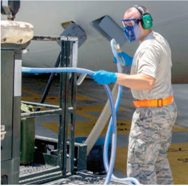
Tech. Sgt. Alejandro Lopez, 735th Air Mobility Squadron non-commissioned officer in charge of aircraft services, prepares to hook a “blue juice” hose up to a C-17 Globemaster III during the de-fleeting process on the Joint Base Pearl Harbor-Hickam flightline Aug. 26. (See additional photo on page A-5.)
