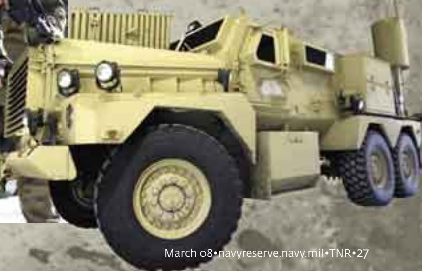
BELOW: The Joint Explosive Ordnance Rapid Response Vehicle. This 42,000-pound vehicle allows explosive ordnance disposal teams to safely travel to and from an incident site and allows them to work inside the vehicle during a call.
