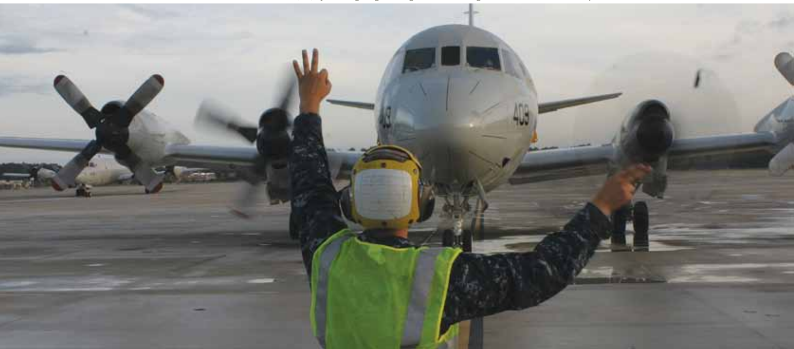
▼ Aviation Machinist's Mate 2nd Class (AW) Tyler Ensign signals engine three turning on a P-3C Orion maritime patrol aircraft.
