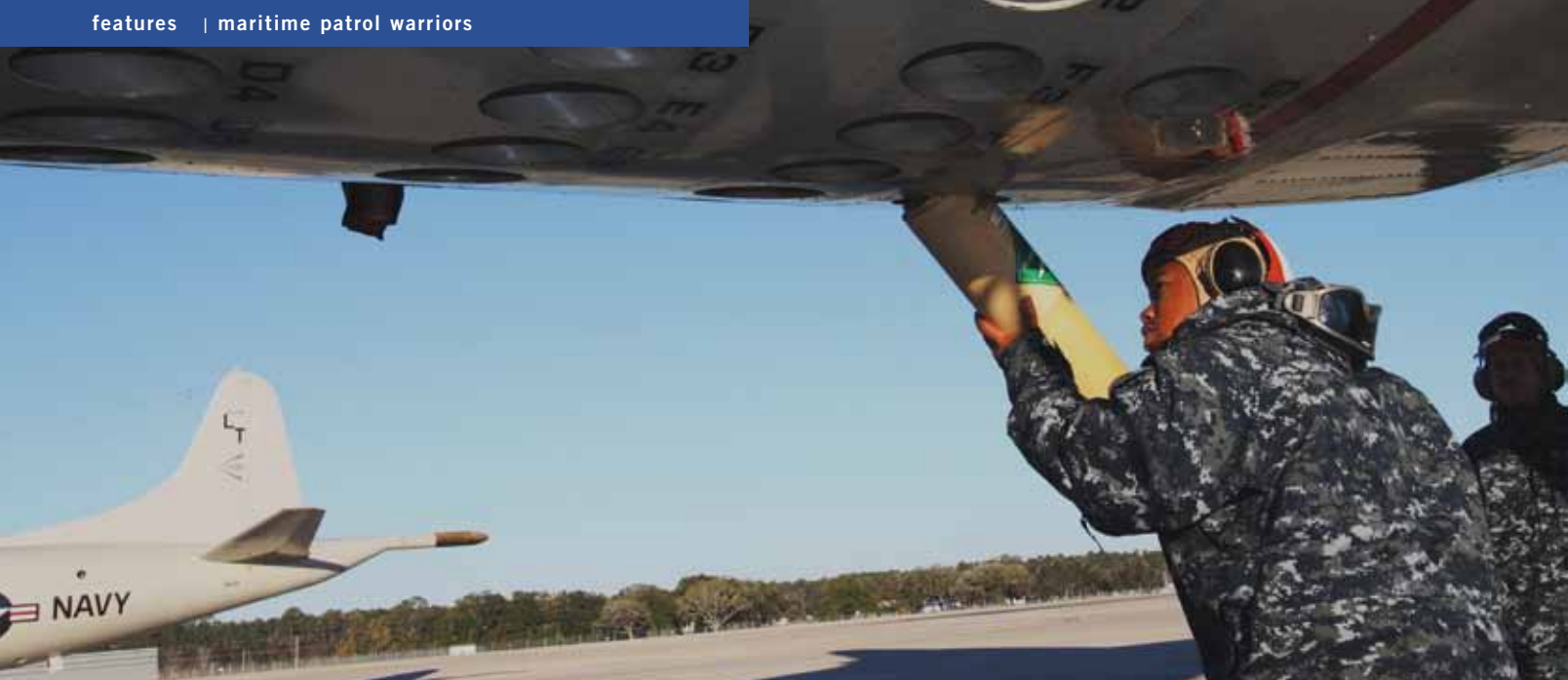
▲ Aviation Ordnanceman 2nd Class Ledarryl Wesley inserts a sonobuoy into one of the sonobuoy launch tubes on the underside of a P-3C Orion maritime patrol aircraft.
