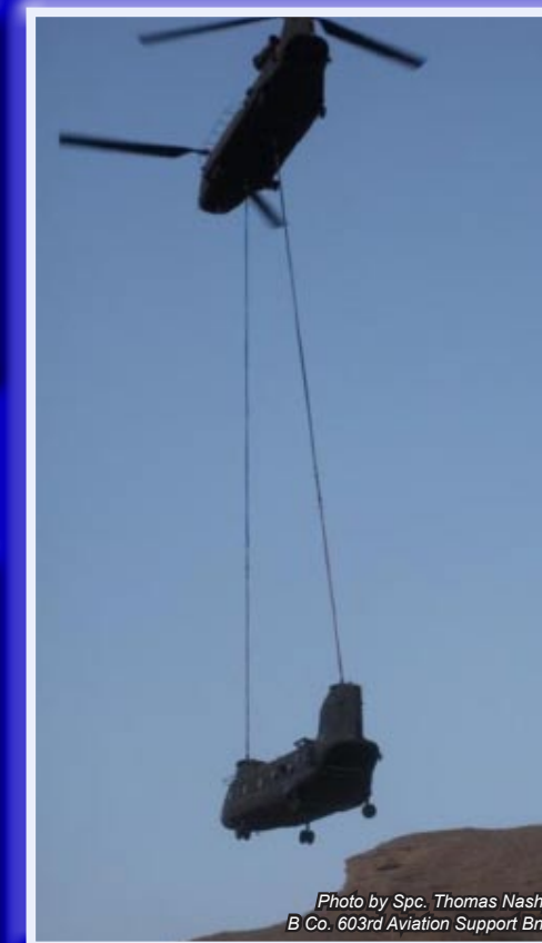
A CH-47 Chinook sling loading another Chinook. It was the first time to happen in Afghanistan. The Chinook had to be sling loaded out due to a blade strike. So the Downed Aircraft Recovery Team went in and prepared the aircraft to be picked up.
