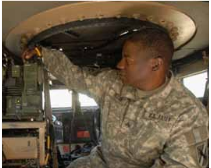
U.S. Army Sgt. Timothy R. Folsom, of Alpha Company Transportation conducts a unscheduled communications check on radios in a vehicle as part of preventive maintenance procedure. Alpha Company Transportation conducts preventive maintenance on their vehicles to ensure their mission readiness. (U.S. Navy photo by Mass Communication Specialist 3rd Class Jeffery M. Richardson/Released)
