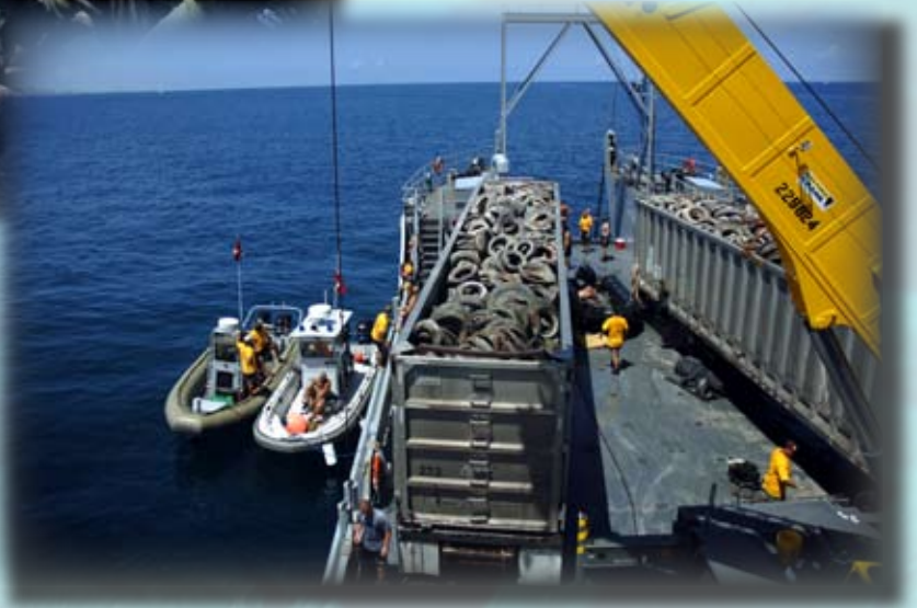
Below: Divers retrieve tires from 70-foot deep waters and string about 80 tires at a time to a metal cable. A "lift bag" is attached to the cable of tires and inflated to bring the tires to the surface.
