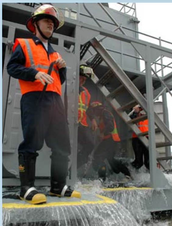
Hospital Corpsman 2nd Class (SW) Bryan Armock demonstrates the hazards of opening a hatch with water behind it.
