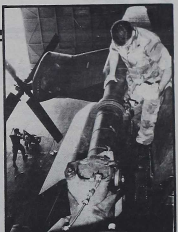
Cpl. John Carr, hydraulics technician for HMH-461, examines the main rotor assembly of a CH-53E 'Super Stallion' for telltale leaks.
