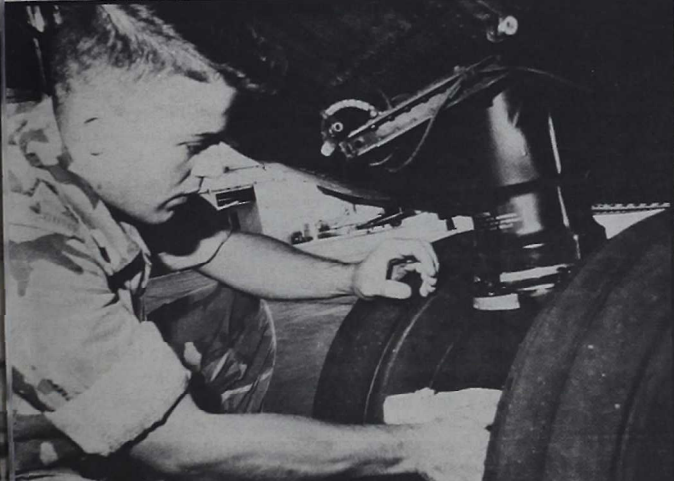
Changing the hydraulic fluid in the landing gear of a CH-53E 'Super Stallion,' John Carr performs a final inspection to insure the system is sealed.
