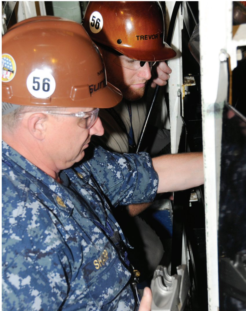
▲ Onboard USS Memphis, Surgemain reservist Chief Machinist Mate Scott Sharp and Shop 56 Pipefitter Trevor Watt work with a Lokring machine which places caps on hydraulic lines.
