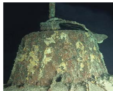
▲ Conning tower of a Japanese mini-submarine showing damage from a shell fired by USS Ward .
