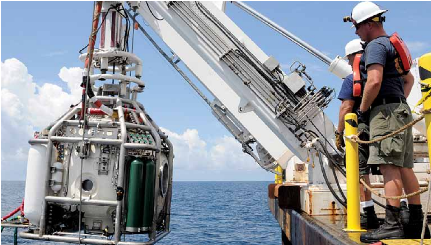
▲ More than 65 miles south of the coast of Panama City Beach, Fla., Navy Diver 1st Class Alvin Carter watches as a massive winch hoists a manned dive bell back from a depth of more than 600 feet of sea water (FSW).
