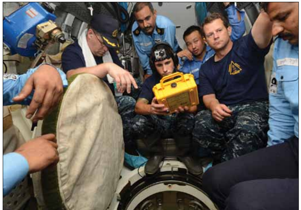
▲ Prospective Undersea Rescue Command Commanding Officer Cmdr. Andrew Kimsey observes Navy Diver 3rd class (AW) John Yarmey take atmospheric readings after opening the transfer hatch of the Pressurized Rescue Module (PRM). U.S. Navy photo by Mass Communication Specialist 2nd Class (EXW) Sebastian McCormack.
