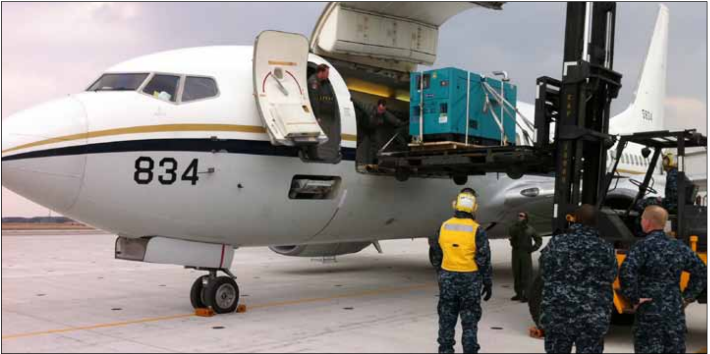
▲ The C-40 Clipper aircraft fulfills the U.S. Navy unique fleet essential airlift requirements by providing medium lift, intra-theater transportation of passengers, cargo or a combination of both. U.S. Navy photo.
