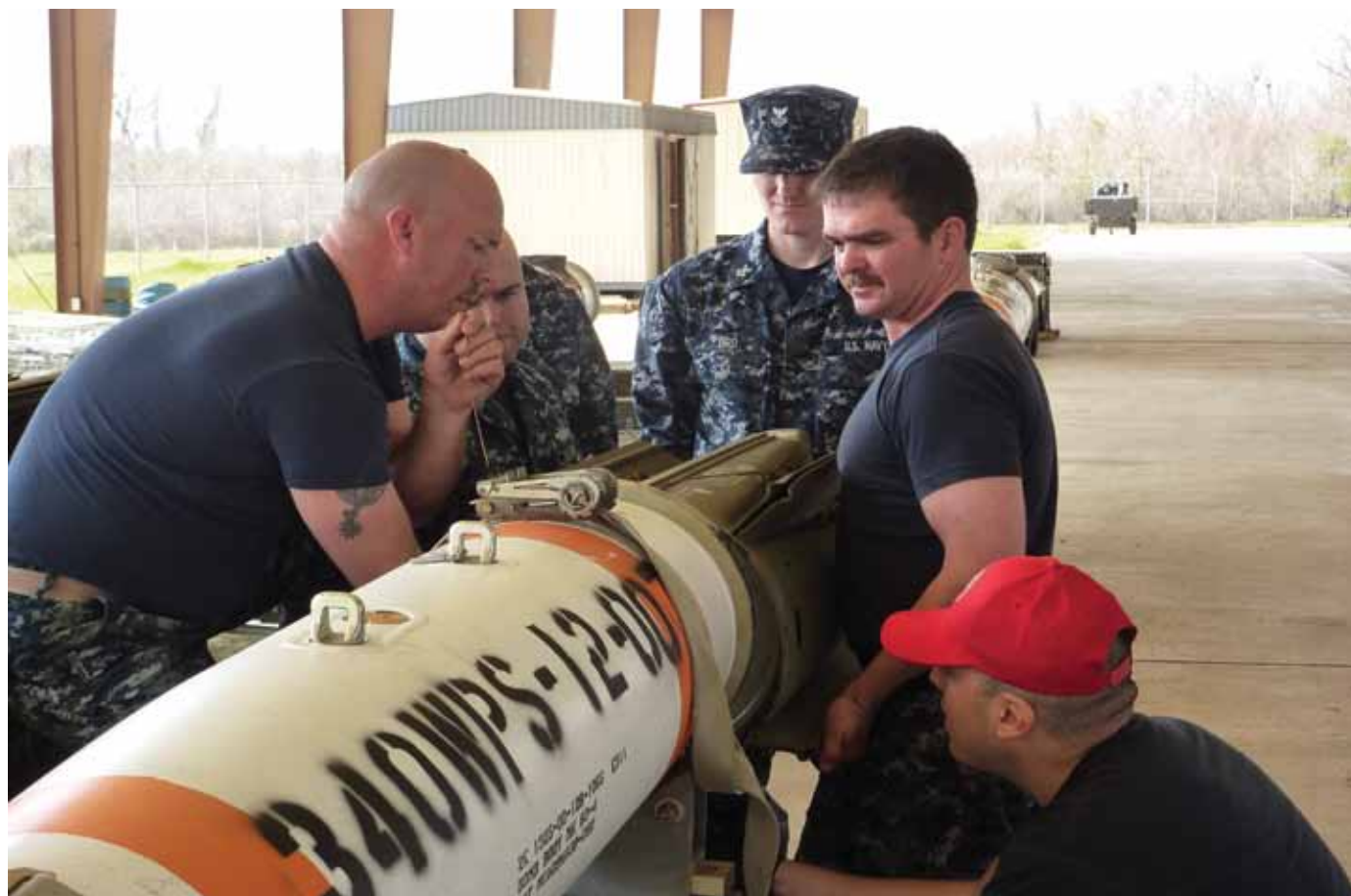
▲ Chief Mineman (SW/AW) John Davis, Gunner's Mate 2nd Class Christopher Corley, Yeoman 1st Class Balance Bird, Mineman 1st Class Scott Landers and Mineman 2nd Class (SW) Frank Alvarado place an MAU- 91 fin assembly on a MK63 training mine. U.S. Navy photo
