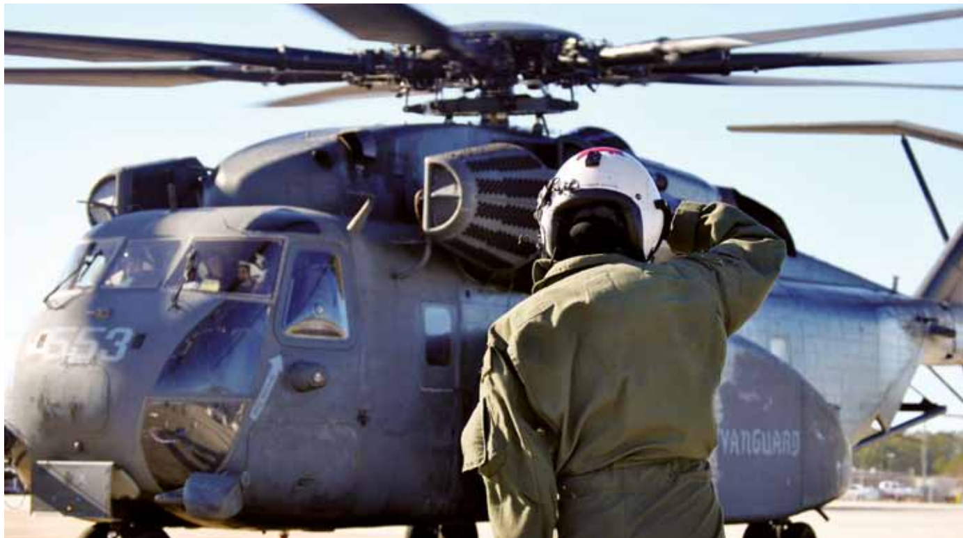
▲ Naval Aircrewman 3rd Class Anastasia Reuwer of Helicopter Mine Countermeasure Squadron (HM) 14 signals the cockpit crew of a squadron MH-53E helicopter during a functional flight check (FCF) following maintenance procedures.
