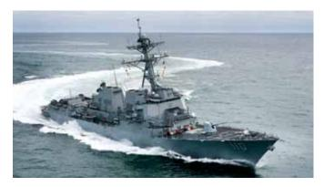
Guided missile destroyers are multi-mission anti-air warfare, antisubmarine warfare, and anti-surface warfare surface combatants. The destroyer's armament has greatly expanded the role of the ship in strike warfare utilizing the MK-41 vertical launch system.
