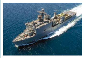
LSD 41 was designed specifically to operate LCAC vessels. It has the largest capacity for these landing craft (four) of any U.S. Navy amphibious platform. It also provides docking and repair services for LCACs and for conventional landing craft.
