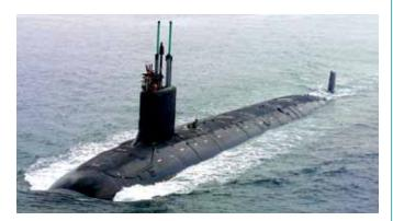
There are three classes of SSNs now in service. Los Angeles class submarines are the backbone of the submarine force with 42 in commission. Thirty-one Los Angeles class SSNs are equipped with 12 vertical launch system (VLS) tubes for firing Tomahawk cruise missiles.
