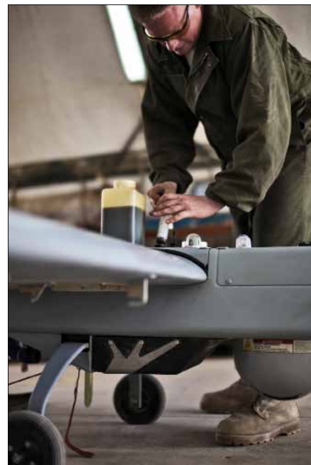
Ensuring the Shadow UAV is ready for the next flight, Spc. Ben Hughes from Fort Drum, N.Y., and a Shadow maintainer assigned to 2nd Brigade Special Troops Battalion, 2nd Bde. Combat Team, 10th Mountain Division, refills the aircraft’s oil reservoir March 7.
