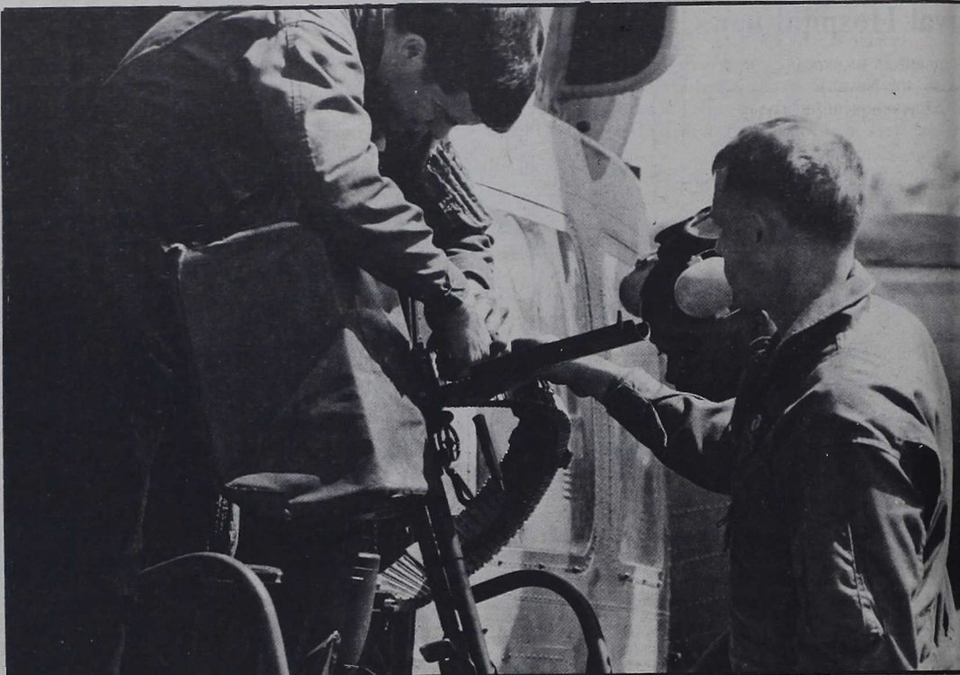
A crew chief and ordnance men mount an M-60 machinegun on a UH-1N Huey. The Huey can also be equipped with 2.5 inch rockets mounted to supplement the teams fire-power.
