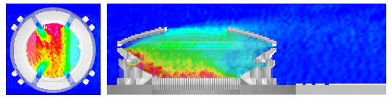
The cadets tested variations in the interior and surrounding flow by altering wind angles from rotating the stadium and using different injection portals with the chemical's dispersion velocity and concentration scans as part of the results.
