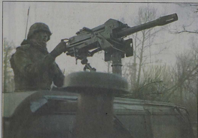
A Marine provides security from atop a High Mobility, Multi-purpose Wheeled Vehicle with a MK-19, 40 mm automatic grenade launcher, near a landing site while other Marines move equipment ashore.
