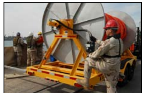
Petty Officer 1st Class Carl M. Sette, machinery technician, Port Security Unit 312, operates the hydraulic control on the oil containment boom to regulate the rate the boom is played out Dec. 14, 2009.
