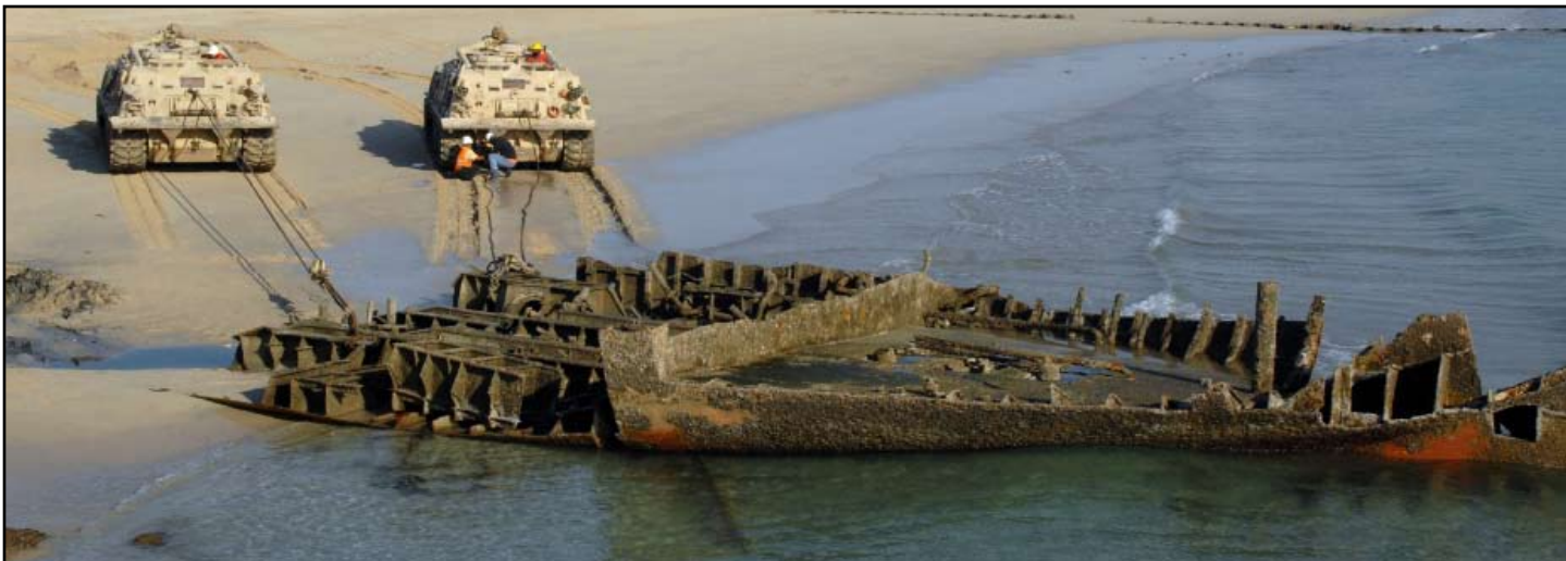
Two M88 recovery vehicles are used to lift the boat out of the sand and water allowing the workers to evaluate the wreckage and see what needs to be done to finish separating the pieces at Camp Patriot, Kuwait, Nov. 11, 2009.
