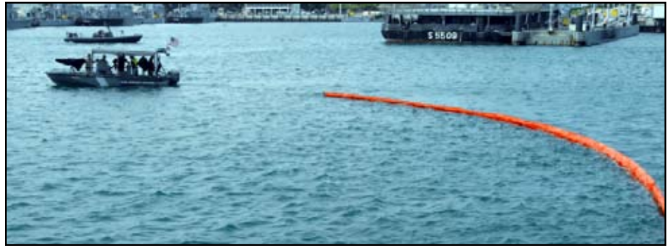
A 25 foot Transportable Port Security Boat manned by Coast Guardsmen from PSU 301 who recently redeploy back to the U.S. and some of their replacements from PSU 312 guide the boom into place which would keep the oil spill floating on the water from spreading until it can be removed.
