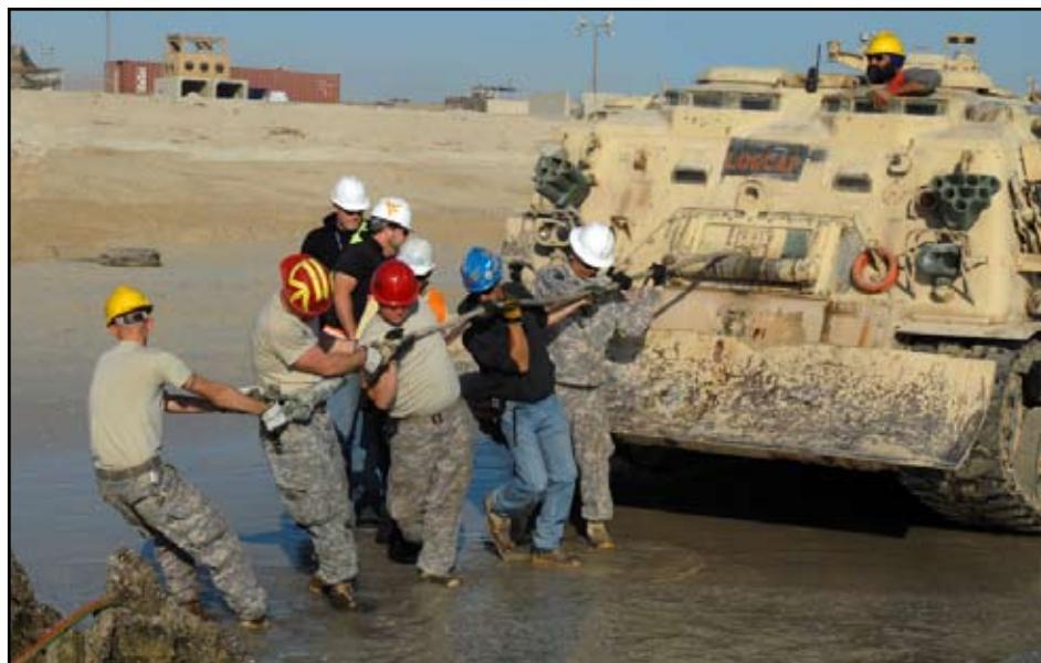
Soldiers from the 1-147 FA along with contractors from DynCorp attach cables from the wenchies on M88 recovery vehicles to the tug boat to pull it from the water.
