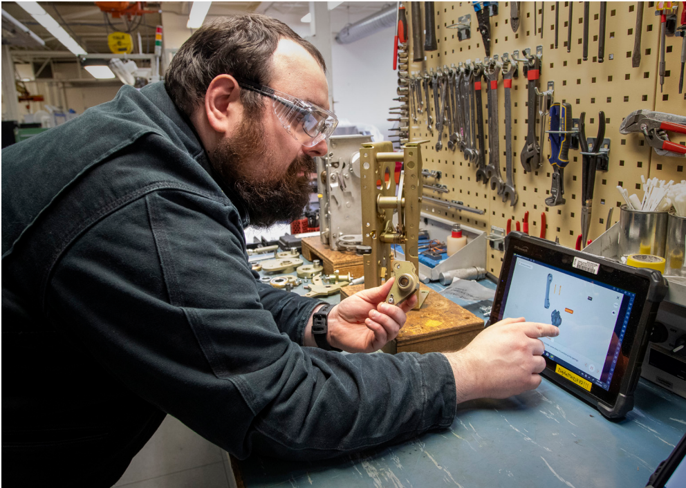
Kevin Vergason, apprentice electrician, Shop 51, Electricians, uses the BILT app on a tablet to build components for a 5-KV circuit breaker. Puget Sound Naval Shipyard & Intermediate Maintenance Facility is piloting this app in the breaker shop with step-by-step work instructions to walk mechanics through the assembly and disassembly of two different breakers. (US Navy photo by Wendy Hallmark)
