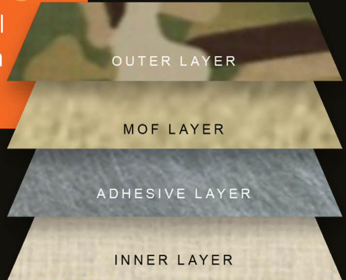
Fabricated laminate swatch contains four layers: Inner layer: soft, high-density knit; Adhesive: thermal glue; MOF layer: MOF-based textile; Outer layer: flexible, tough, flame-resistant material. (NuMat Technologies photo)
