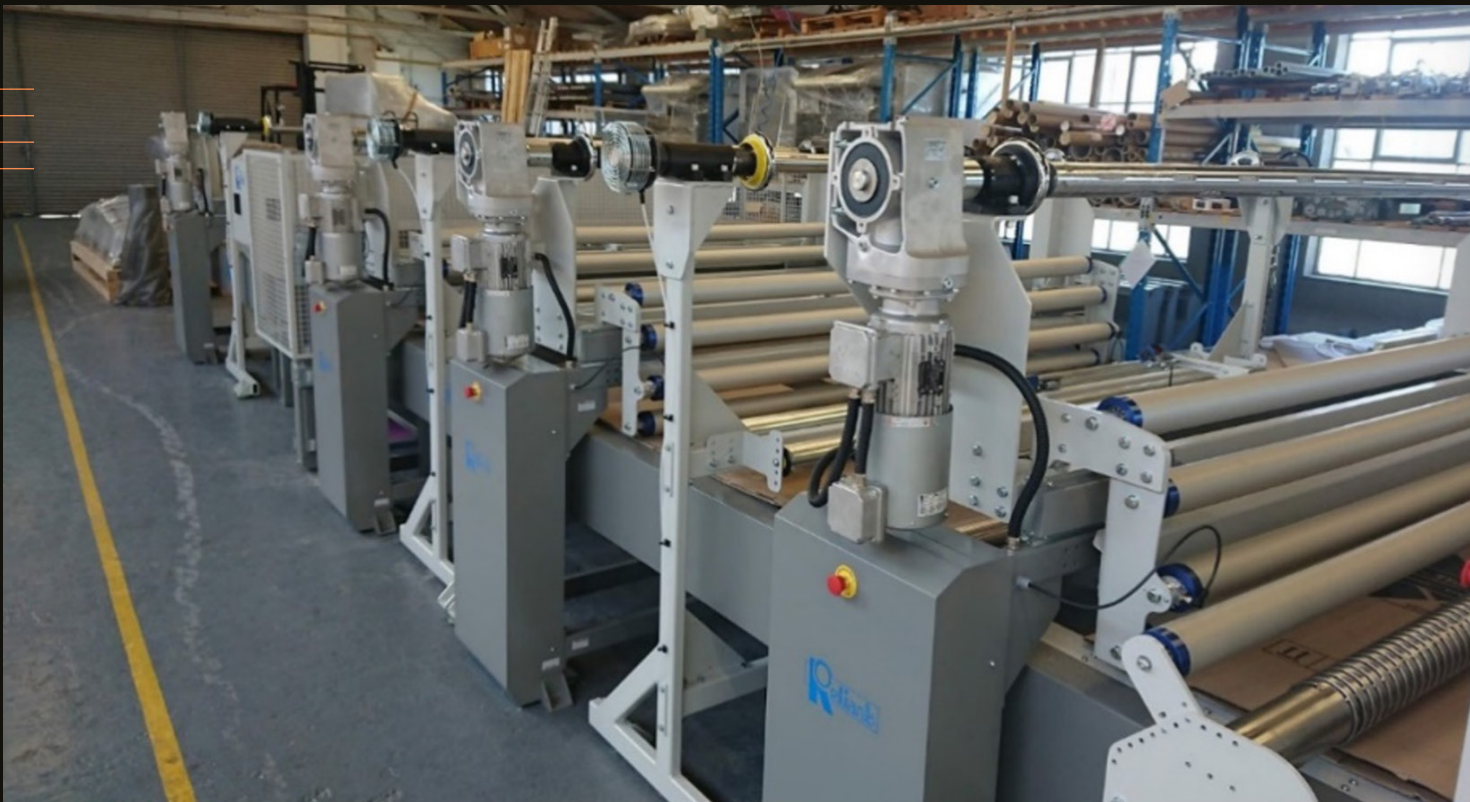
This fabrication floor allows roll-to-roll manufacture of laminated textiles that contain zirconium hydroxide for prototype protective garment design. (Guild Associates photo)
