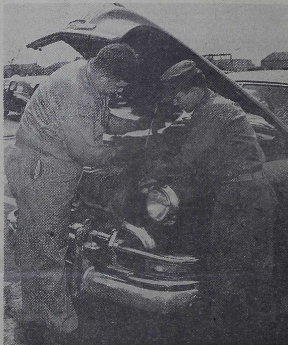
HELPING HAND —Cpl. Clyde T. Guthrie, left, helps Pfc Scheiman, "A" Co., 2nd Engineer Bn., replace burned-out brushes in his automobile generator.
