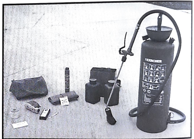
(Above) From left to right: detection paper, Draeger tube set, carrying pouch (in back), individual-decontamination kit, vehicle-decontamination kit, and backpack sprayer (Below) A student secures his mask before removing his jacket.
