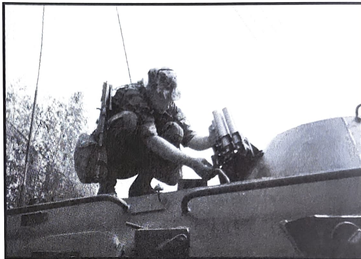
Loading signal flares into the BTR-80 RhM-4, part of precombat checks on the vehicle
