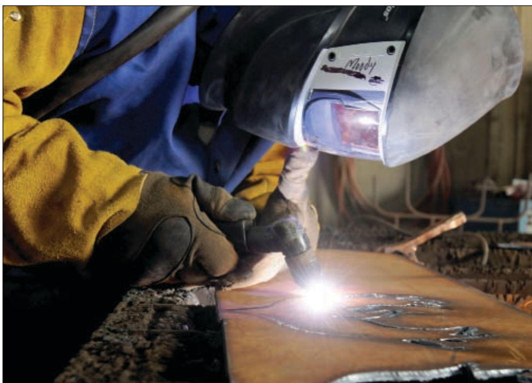
Pfc. Benjamin Moody, a metal worker with the 546th Maintenance Company, 732nd Combat Sustainment Support Battalion, 36th Sustainment Brigade, 13th Sustainment Command (Expeditionary) and a Green Cove Springs, Fla., native, uses a plasma torch to cut metal plates March 6 at Contingency Operating Base Adder, Iraq.
