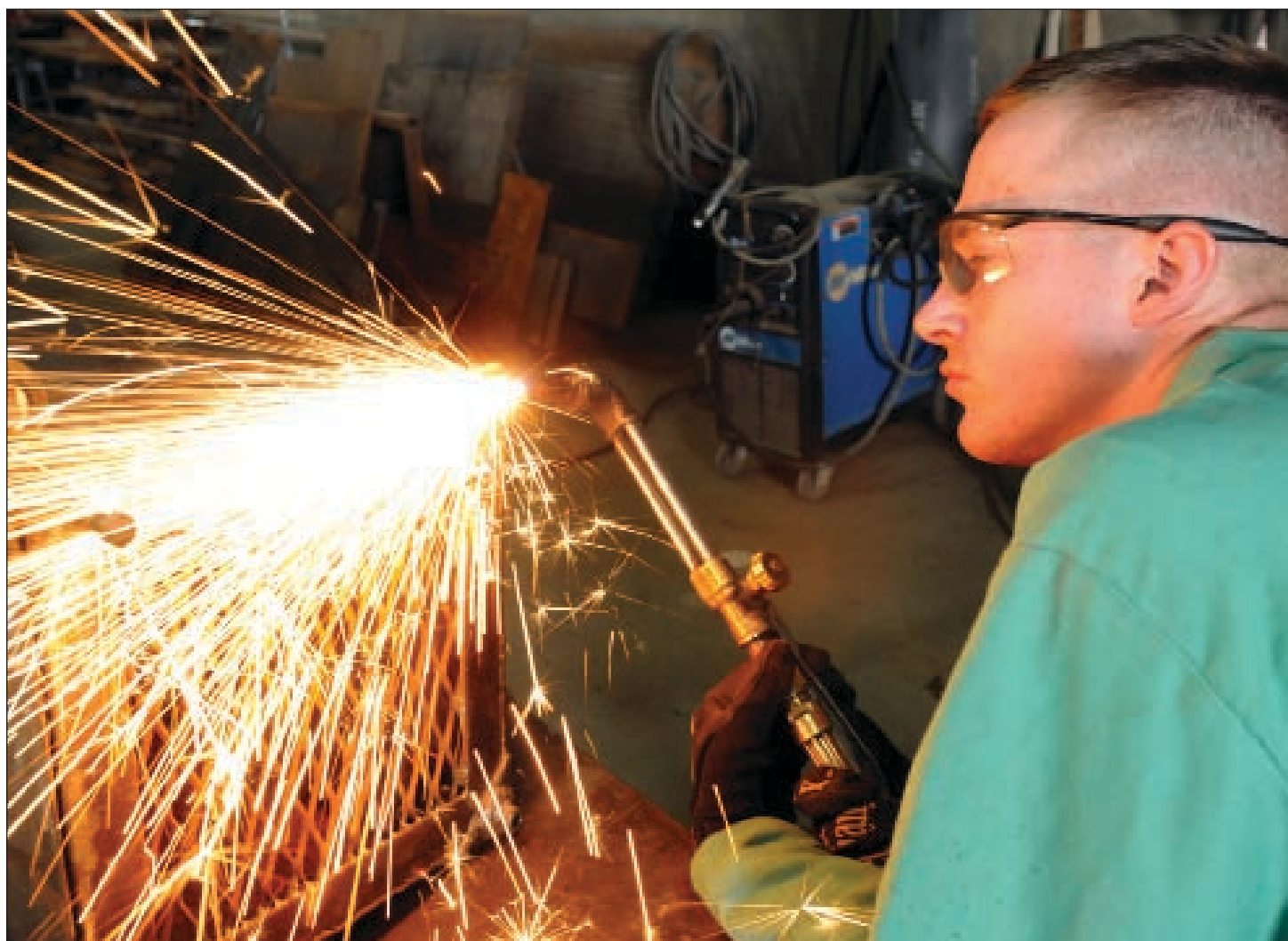
Spc. Nathan Mast, a metal worker with the 546th Maintenance Company, 732nd Combat Sustainment Support Battalion, 36th Sustainment Brigade, 13th Sustainment Command (Expeditionary) and a Grand Rapids, Mich., native, uses a cutting torch while fabricating a toolbox March 6 at Contingency Operating Base Adder, Iraq.
