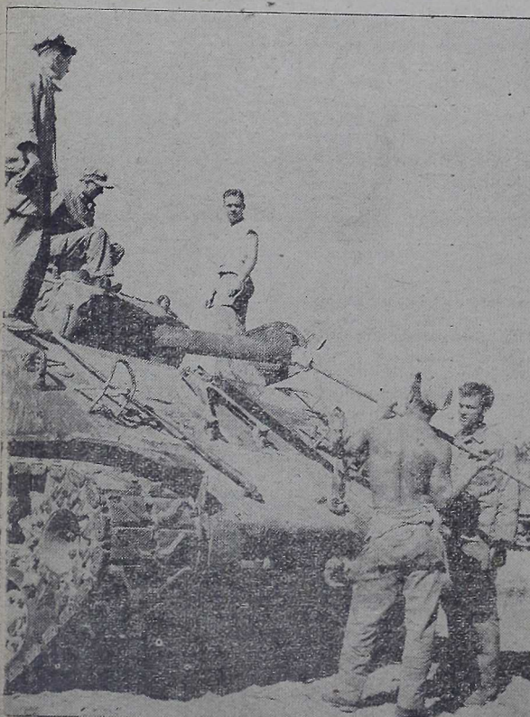
It's not quite the same as an M-1, but it still has to be cleaned. Crew members of the tank turn to on the 105mm Howitzer after a hard day in the field. The gun is only one of the many details which demand constant attention if the tanks are to operate properly. (All photos on this page by Cpl. Pajakowski, 2d Division Photo Section.)
