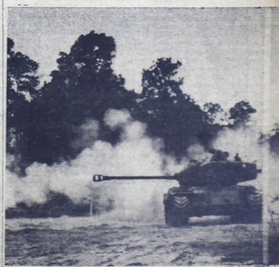
An M-26 tank fires its 90mm rifle during training exercises of the Second Tank Bn., Second Marine Division (Photo by Sgt. Albert Greenwell).
