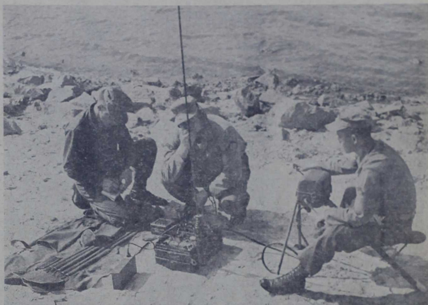
DURING AN EXERCISE, students in the Field Radio Operators course, set up an AN/GRC-9 portable field radio to transmit messages to posts in the woods several hundred yards away. The course teaches men the operation of all the field radio
