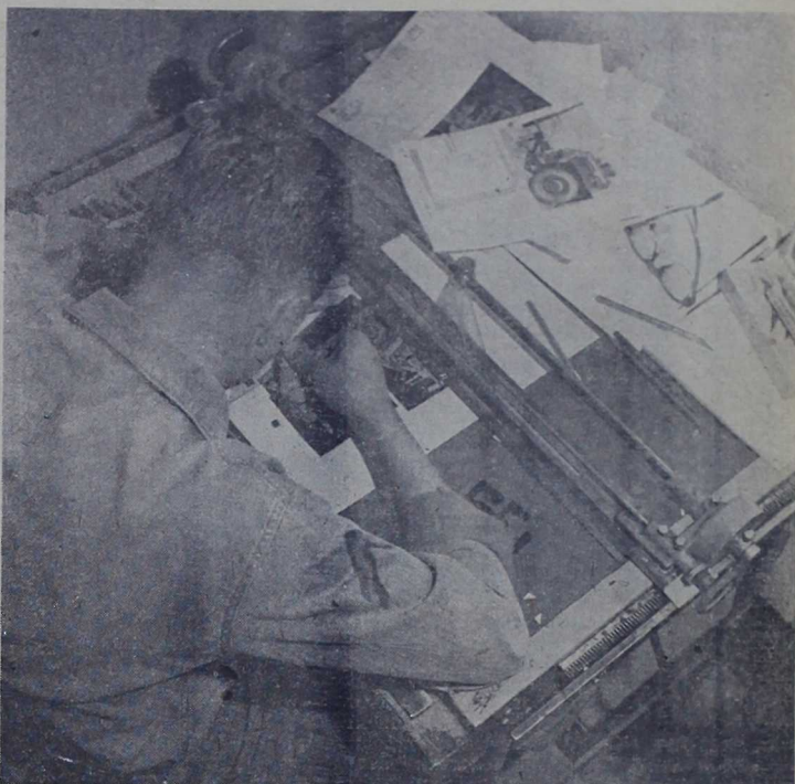
THE NEGATIVE is placed on a light-table and stripped, mounted and "opaqued" by a copy layout man like Cpl. Joe Orel Jr. Orel paints out clear spots on the negative and tapes in a file number that allows the plant to keep track of each job at a glance . . .
