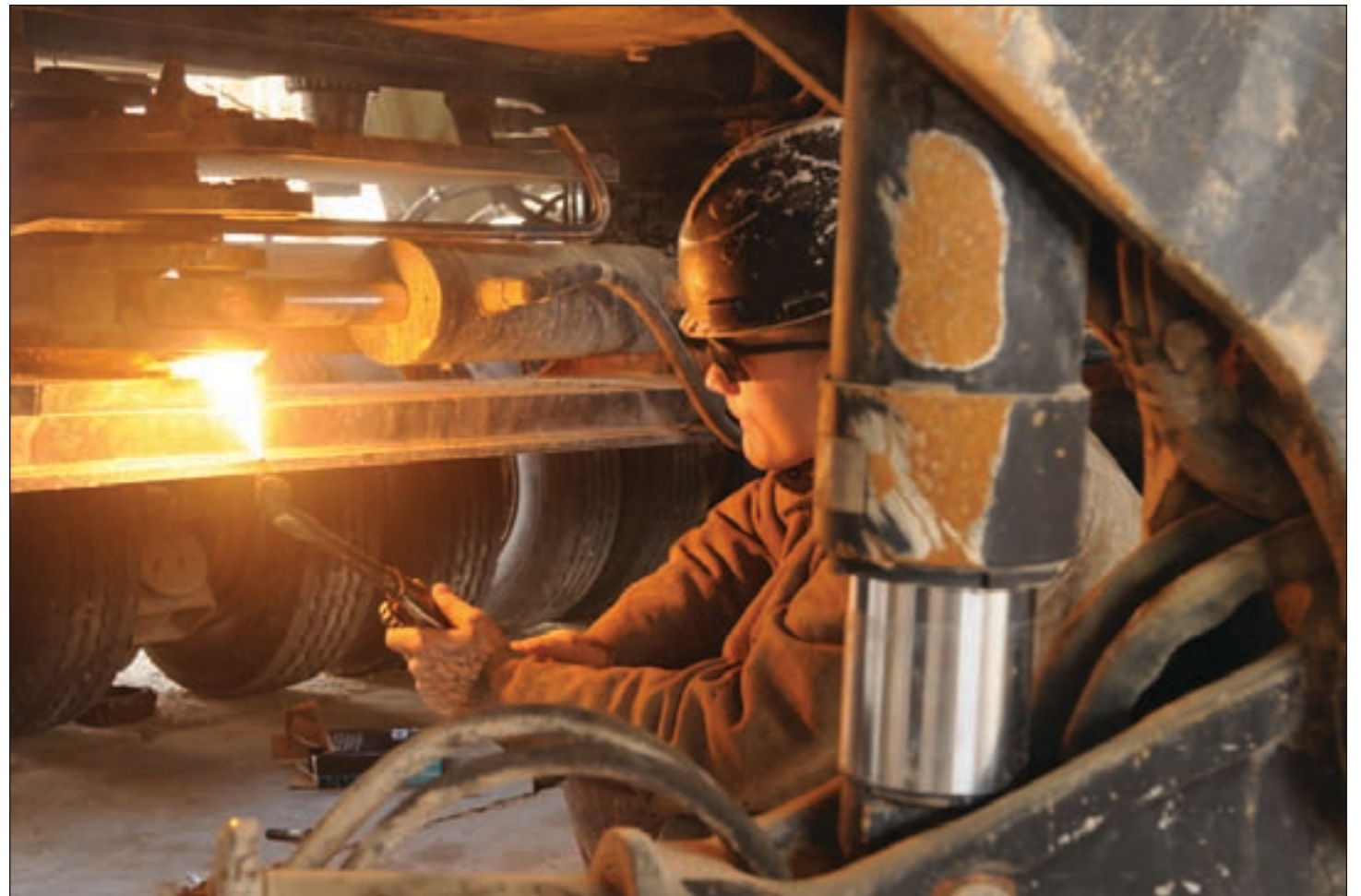
Spc. Scott Gordon, a Heavy Equipment Transporter system mechanic with the 514th Support Maintenance Company, 80th Ordnance Battalion, 15th Sustainment Brigade, 13th Sustainment Command (Expeditionary) and a Fort Lewis Wash., native, uses a blow torch to perform maintenance on a steering component of a HET Feb. 24 at Joint Base Balad, Iraq.
