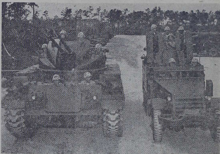
TRIPLE-THREAT STARS on the AAA team are these two mobile gun carriages manned by their squads. Labeled the M-42, at left, which carries "twin 40s", and the M-16 with four air-cooled 50 cal. machine guns.
