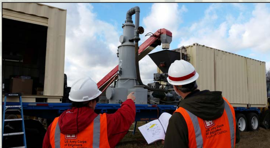
USACE works at Camp Ravenna, Ohio, on a pilot study to treat contaminated soils using a Vapor Energy Generator.
