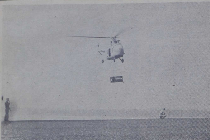
DROP —Compact battalion aid station is set down by an HRS helicopter during demonstration for 2nd Marine Division officers.
