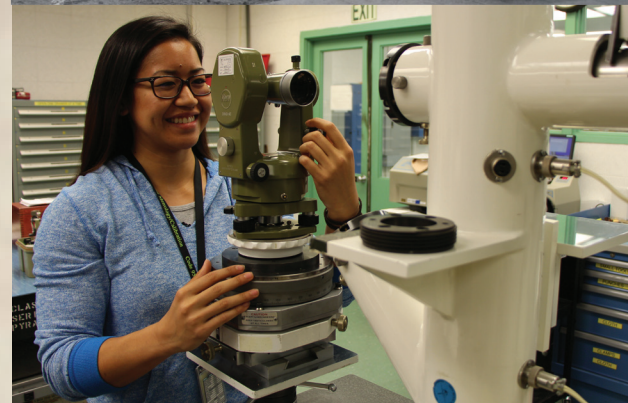
Shop 67 Calibrations Apprentice Noelani Mikami is looking through a Kern Theodolite. It is a precision instrument used for measuring angles in the horizontal and vertical planes. Photo taken in April 2017.
