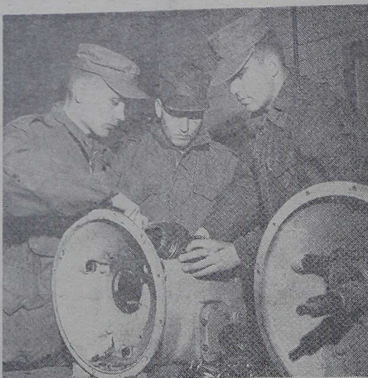
FROM ALL POINTS — Motor Transport students represent every Marine Corps post and station. Shown here disassembling a five-speed transmission are Cpl. Stonewall Taylor, MCAS, Miami, Fla., left, Cpl. James L. Tait, MCAF, Santa Anna, Calif., center, and Cpl. D. F. Grunde, Pickle Meadows, Calif.
