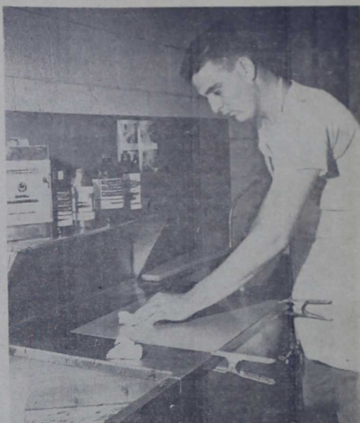
PREPARING PLATE —Sgt. Kenneth W. Edwards develops the image of the printing matter on a pre-sensitized metal plate. The plate, which functions much the same as a mimeograph stencil, is placed on an offset press to reproduce the required amount of copies.
