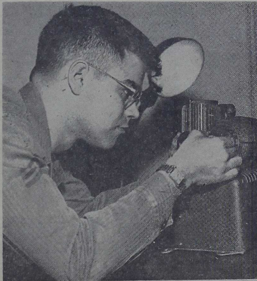
PROJECTOR TECHNICIAN —Act. Sgt. Karl W. Staiger, sound equipment repairman, replaces a worn armature in a 16mm projector.
