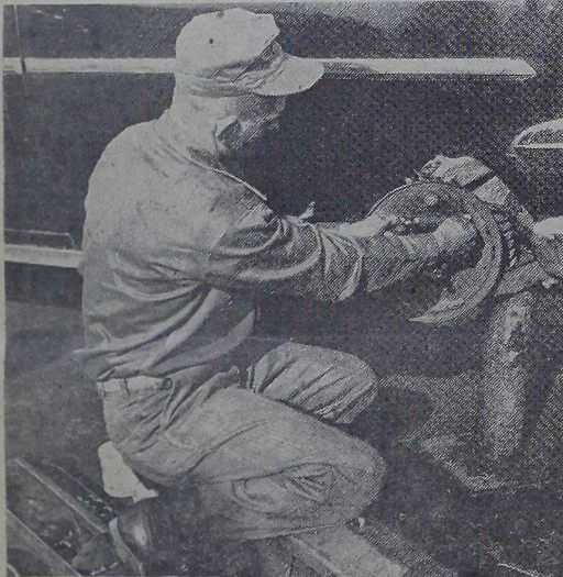
BRAKE REPAIR —Pfc Edward A. Tremblay found he could replace his brake-linings much more economically by using facilities at the Base Automotive Hobby Shop.
