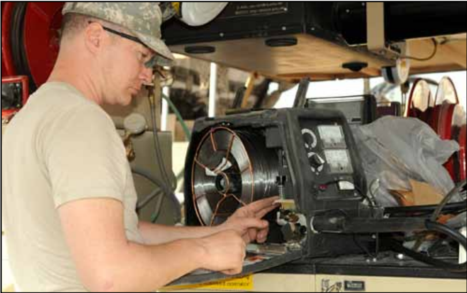
Sgt. Christopher Noguera, a mechanic assigned to Company B, puts additional wire into a welder in preparation for a welding project.
