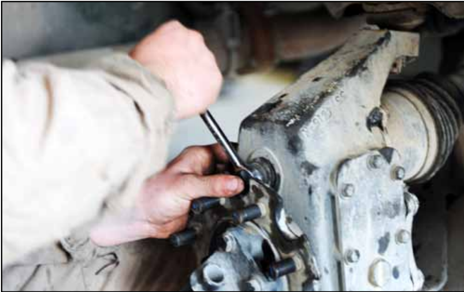
During an annual servicing, Pfc. Zachery Padon, a mechanic assigned to Company B, checks the integrity of the steering linkage on a humvee Jan. 21.
